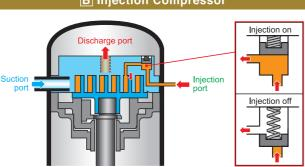
Effect: Improves heating capacity at low outdoor temperatures, and enables higher outlet temperature adjustment and
