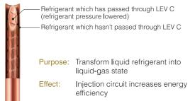
The compressor is subjected to a heavy load when compressing liquid refrigerant, and the result is lower operation efficiency. The addition of HIC supports refrigerant heat exchange at two different pressure levels. The heat-exchange process transforms the injected liquid refrigerant into a gas liquid state, thereby decreasing the load on the compressor during the compres-
