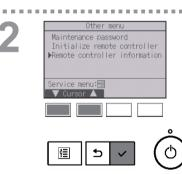
Move the cursor to "Remote controller information" with the F1 or F2 button, and press the SELECT button.
