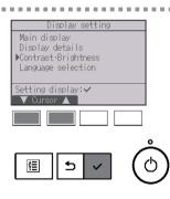
Move the cursor to "Contrast-Brightness" with the F1 or F2 button, and press the <u>SELECT</u> button.
