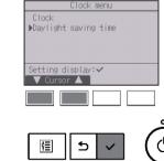
Move the cursor to "Daylight saving time" with the F1 or F2 button, and press the <u>SELECT</u> button.
