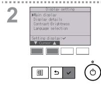
Move the cursor to "Main display" with the F1 or F2 button, and press the SELECT button.
