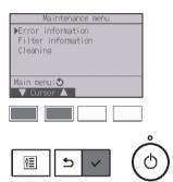
To display the error information screen, select "Error information" from the Maintenance menu. Errors cannot be reset.
