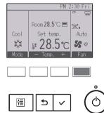
Each pressing of the  $\boxed{F4}$  button cycles through the following fan speeds.
