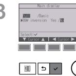
Select "B&W inversion" with the F1 or F2 button, and select the display mode "Yes" or "No" with the F3 or F4 button, and press the SELECT button. (The factory setting is "No.")
