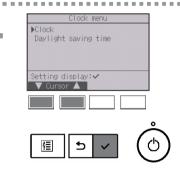
Move the cursor to "Clock" with the F1 or F2 button, and press the SELECT button.
